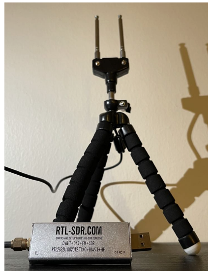
Figure 1. SDR RTL2832U and antenna used in PRF data collection.
