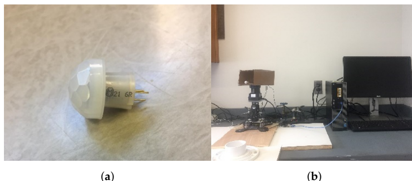
Figure 2. (a) The Panasonic AMN 24112 PIR sensor and (b) the complete MI-PIR system.
