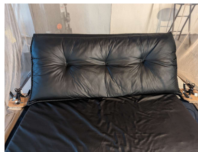
Fig. 6. The setup for human subject data acquisition inside the shield. Two SDR devices were fixed on either side of the human subject and pointing to the human subject.
