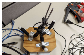
Fig. 4. RTL-SDR device used in the experiment.
